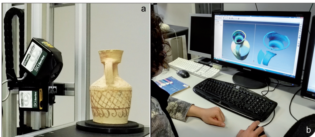
Fig. 2. 3D scanning (a) and modelling of an artifact (b).
